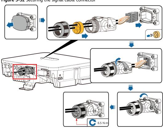
Figure 5-32 Securing the signal cable connector
