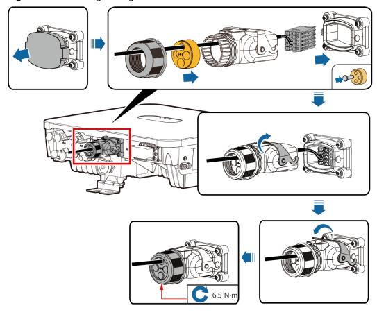
Figure 5-34 Securing the signal cable connector
