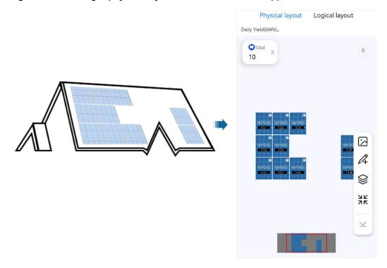
Figure 7-4 Viewing a physical layout on the FusionSolar SmartPVMS
