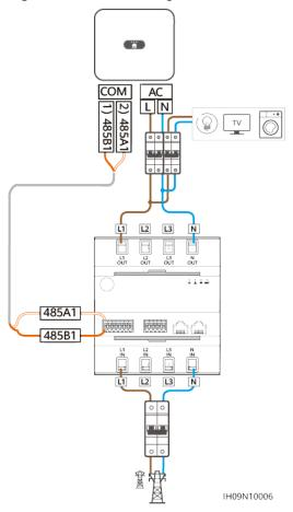
Figure 5-21 Connecting cables to the EMMA
