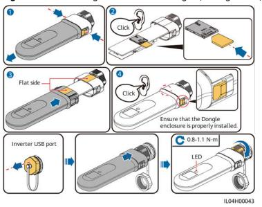
Figure 5-37 Installing the 4G Smart Dongle (SDongleB-06)
