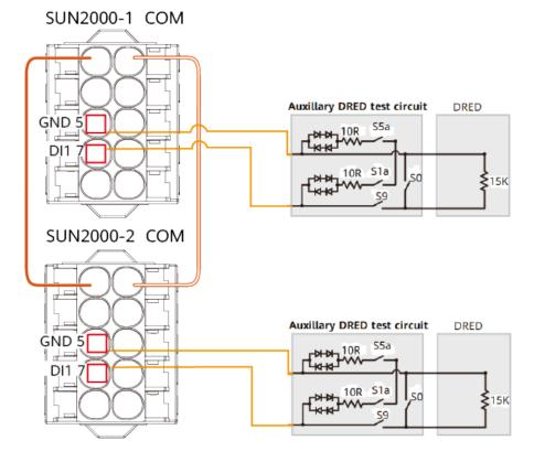
The demand response enabling device (DRED) is a power grid dispatch device.
