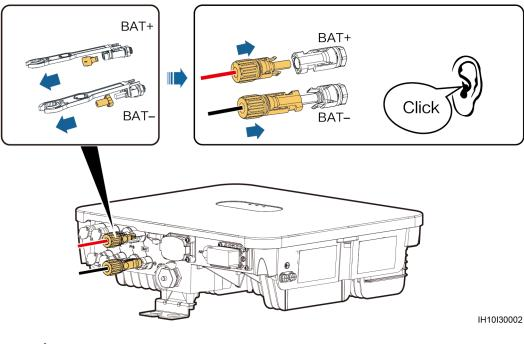
Figure 5-12 Connecting battery cables
