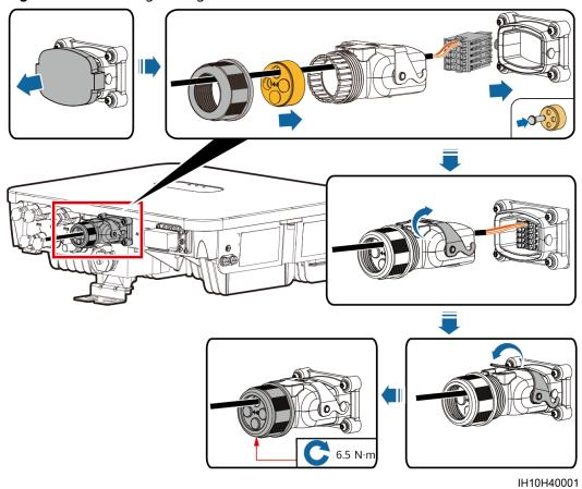
Figure 5-20 Securing the signal cable connector
