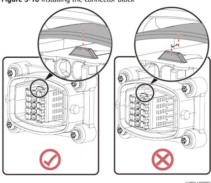
Figure 5-18 Installing the connector block
