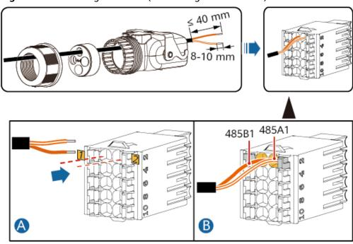
Figure 5-22 Installing the cable (connecting to the EMMA)
