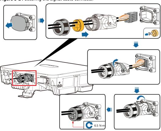
Figure 5-24 Securing the signal cable connector
