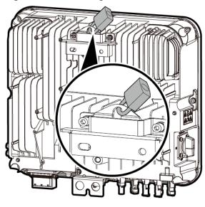
Figure 4-10 Installing an anti-theft lock
